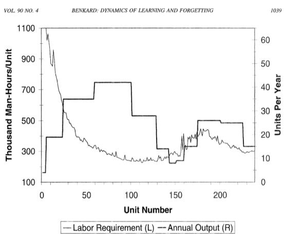
FIGURE 1. L-1011 PRODUCTION: DIRECT LABOR REQUIREMENT AND YEARLY OUTPUT
